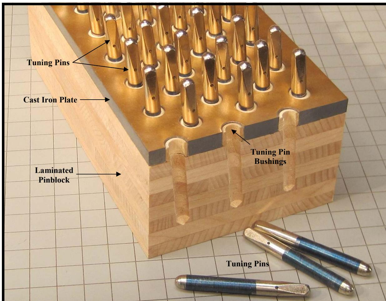
The above cut-away model of a piano pinblock, plate and pins illustrates the origin of the problem. The pinblock is made hardwood, in this case hard rock maple. Its laminations run cross grain to each other to prevent splitting, and to better hold the tuning pins. The pinblock is not ordinarily visible, but is hidden beneath the cast iron plate, which is necessary to hold the tremendous tension on the strings, measuring anywhere from 18 to 20+ tons for the piano as a whole..
