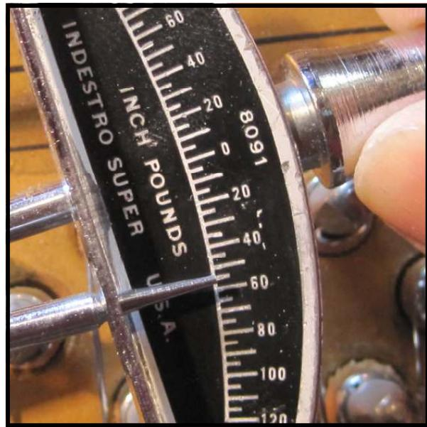
The above photos show torque reading measurements done on the same tuning pin before and after CA glue was administered. In the photo on the left, the untreated pin measures just under 20 inch pounds of torque. After a single treatment the pin measures a much better reading of 55 inch pounds of torque.
