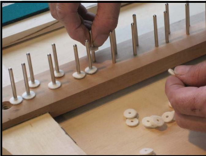
Secondly, while the keyframe is out of the piano, it is an ideal time to consider having the old back rail cloth, balance rail punchings and front rail punchings replaced with new. These felts cushion the keys and help the keys operate silently. Many times the old cloth is either worn out or has been damaged by moths or mice, both of which have a fondness for felt.
