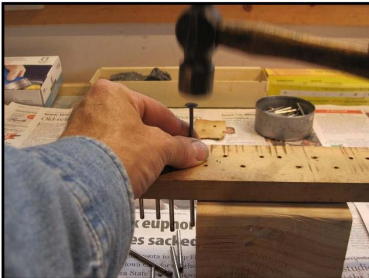
In the photo to the left, balance rail pins are shown being tapped out from the underside of the balance rail. Again, care is taken not to damage the original hole. The old pins will be measured with a micrometer to determine their exact size. The new pins, when they are driven in, will be tight as long as care has been taken in removing the old pins.
